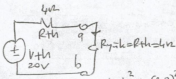
$$P_{max, R_{yük}} = \frac{V_{th}^2}{4R_{th}} = \frac{(20)^2}{4 \cdot 4} = \frac{20 \cdot 20}{4 \cdot 4} = 25 \text{ W}$$
